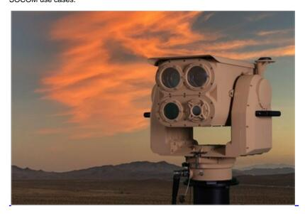
The Viasat Mercury solution is an expeditionary, high-capacity FSOC link with an automated pointing, acquisition, and tracking (PAT) system, offering military operators lower signature communications at the quick-halt. Mercury is based upon advanced commercial-off-the-shelf technology, leveraging substantial industry investment towards bringing a high-performance, resilient, and cost-effective capability to better support warfighting operations at the edge.
