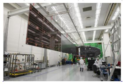
During the integration process, the solar arrays, reflectors and other items were attached to the satellite, bringing it to its full, flight configuration for the first time. The satellite's reflectors will be some of the largest ever sent to space, along with its solar arrays, each featuring eight panels with an overall wingspan of 144 feet, similar in size to that of a Boeing 767 airliner.
